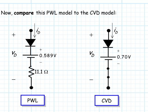
Note that the CVD model can be viewed as a PWL model with  $V_{D0}$  = 0.7 V and  $r_d$  = 0.0. Compare those values with our model ( $V_{D0}$  = 0.589 V and  $r_d$  = 11.1 $\Omega$ )—not much difference!
